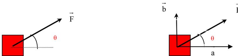
The vector triangle showing the force  $\vec{F}$  and its component vectors  $\vec{a}$  and  $\vec{b}$  is shown below.
