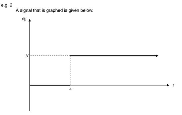
Determine the Laplace transform of the above signal.
