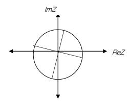
NB: The solutions of  $z^n = rcis\theta$  lie on a circle with centre the origin and radius  $r^{\overline{n}}$  and they divide the circle into arcs of equal length. The symmetrical nature of the solutions can be used to find all solutions if one is known.
